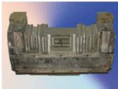
Part of the mould for railway inductors
